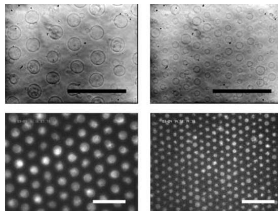
**Figure 2.** Phase-contrast (top) and Fluorescence (bottom) microscopy images of liposomes formed on the lipid pattern after 2 hours of electroswelling (2V, 10 Hz). The lipid patterns consisted of hexagonal arrays of lipid dots having a diameter of 30  $\mu\text{m}$  (left) and 15  $\mu\text{m}$  (right), respectively. Liposomes are made fluorescent by the use Rhodamine-Phosphatidylethanolamine, a fluorescent lipid. For each picture, scale bar is 200  $\mu\text{m}$ .
